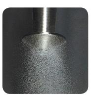
Tight control of drop size is critical to bioaerosol testing processes. The frequency of the ultrasonic nozzle used and the concentration of the liquid being atomized determine the size of dry particles.
