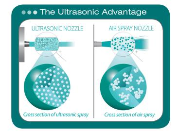
Compared to air spray nozzles, ultrasonic nozzles have the ability to break up any agglomerations of suspended particles when spraying nanosuspensions, due to the ultrasonic vibration of the nozzle.
