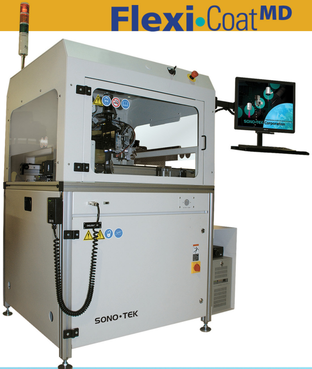
Standalone inline programmable coating system 500x500x100 mm range of motion
